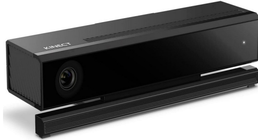
Figure 3.1: Microsoft Kinect v2 sensor for Windows.
