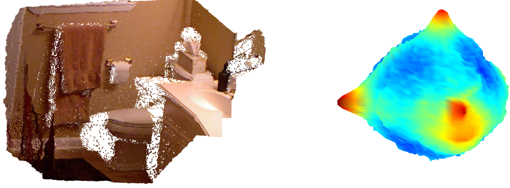
Figure 2.7: Figure (a) shows a scene plotted in 3D Cartesian coordinates, besides it, in (b) a plot of the concentration of normals is shown. It is created using a histogram of the normals, where the concentrations are plotted on a sphere, corresponding to the direction of the normals. Notice the three main bulges (red colors), they correspond to the three dominant normal directions in the image. (In the plotting of (b), the concentration is dampened to make it easier to visualize).
