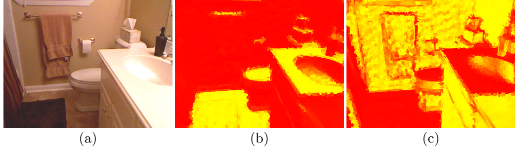
Figure 2.9: The original image is shown in (a). (b) shows the floor probability evaluated using equation 2.6, which has a high value when the surfaces are near parallel with the floor normal direction and low values otherwise. (c) shows a similar feature as (b) for the walls.
