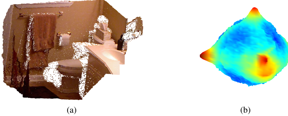
Figure 3: (a) Shows a scene plotted in 3D Cartesian coordinates, besides it, in (b) a plot of the concentration of normals is shown, it is created using a histogram of the normals, where the concentrations are plotted as elevations on a sphere, corresponding to the direction of the normals. Notice the three main bulges (red color), they correspond to the three dominant normal directions in the image.
