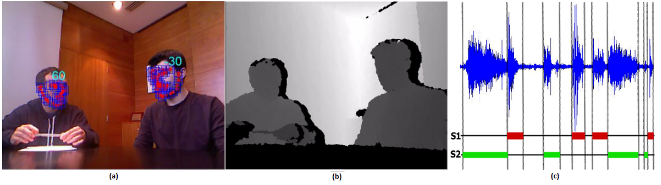
Figure 2: Example of the conversation scenario. Image (a) shows the RGB image with both face detection and head pose estimation. Image (b) shows the corresponding depth map, where the gray hues indicate the distance respect to the camera. Image (c) illustrates the speech diarization process for each subject S1 and S2, where clusters that belong to each one are obtained from the input signal estimating the speech time of each segment, as well as the speech pauses/interruptions.
