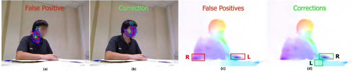
Fig. 6.6 Examples of how the semi-automatic heuristic procedure of [125] works on two pairs of frames of a session. The correction of false positives is shown, improving the continuity of the detection of positive regions of interest between consecutive frames. Image (a) shows a false positive detection for the face region, whereas image (b) shows its correction with the proper fitting. Image (c) shows false positive detections for the hand regions, choosing those blobs obtained by means of skin segmentation having highest optical flow with respect to the previous frame. Image (d) shows the correction of these regions by comparing them with the positive hand detections, recovered from the previous frames.
