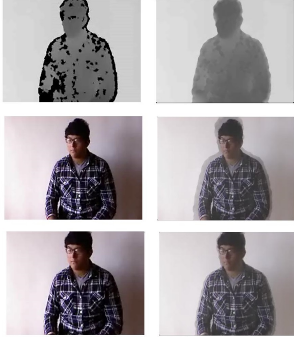
Figure 4.2: 1st row: inpainting+HMF results of a depth sample from isoGD [Wan+16a] dataset. 2nd row: superposition before registration. 3rd row: superposition after registration.
