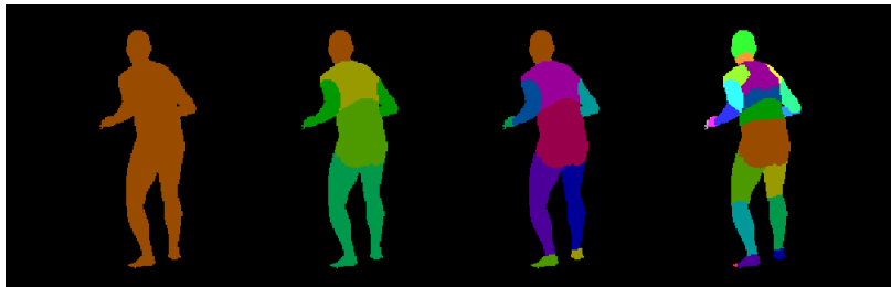
Figure: 1st Experiment , different ground truth resolutions, one for each module. The idea is to learn a progressive refinement of the real ground truth.
