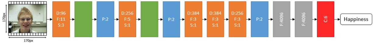
Fig. 4: Single Frame architecture: Orange, green, blue, gray and red boxes indicate convolutional, normalization, max pooling, fully connected and softmax classifier layers respectively.
