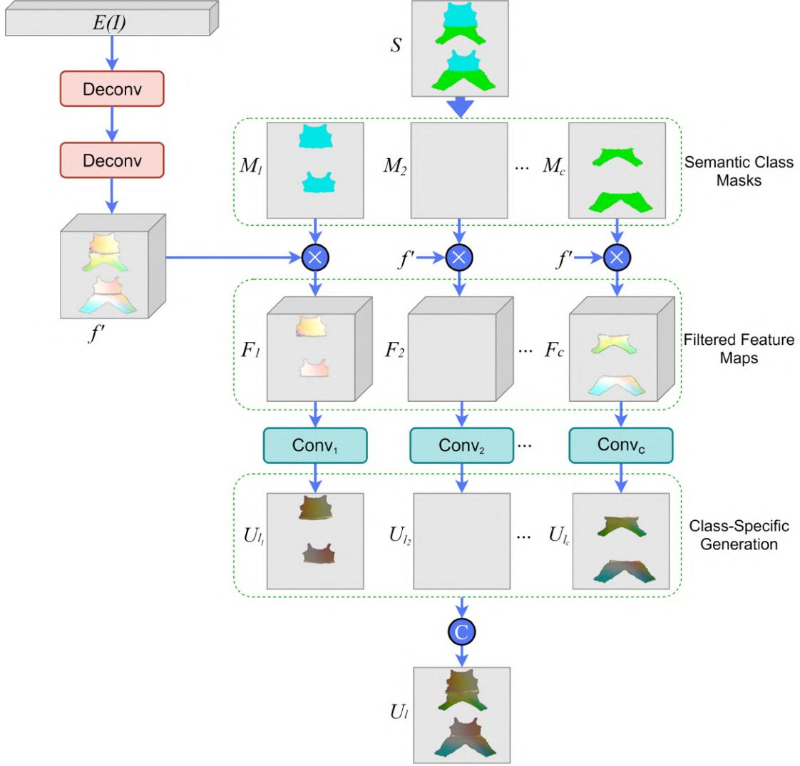
Figure 4.6: Class-Specific Local Generation Network overview. The symbol  $\otimes$  denotes element-wise multiplication, and  $\oplus$  channel-wise concatenation. Source: Own elaboration adapted from [56].
