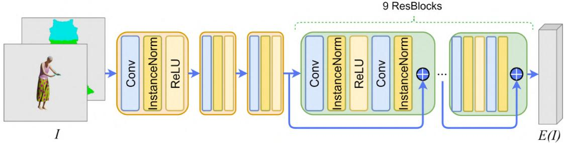
Figure 4.5: Parameter-Sharing Encoder architecture. Contains three convolution blocks and nine residual blocks. Source: Own elaboration.
