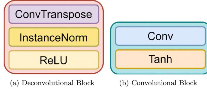
Figure 4.7: Architecture of the deconvolutional and convolutional blocks. Source: Own elaboration.
