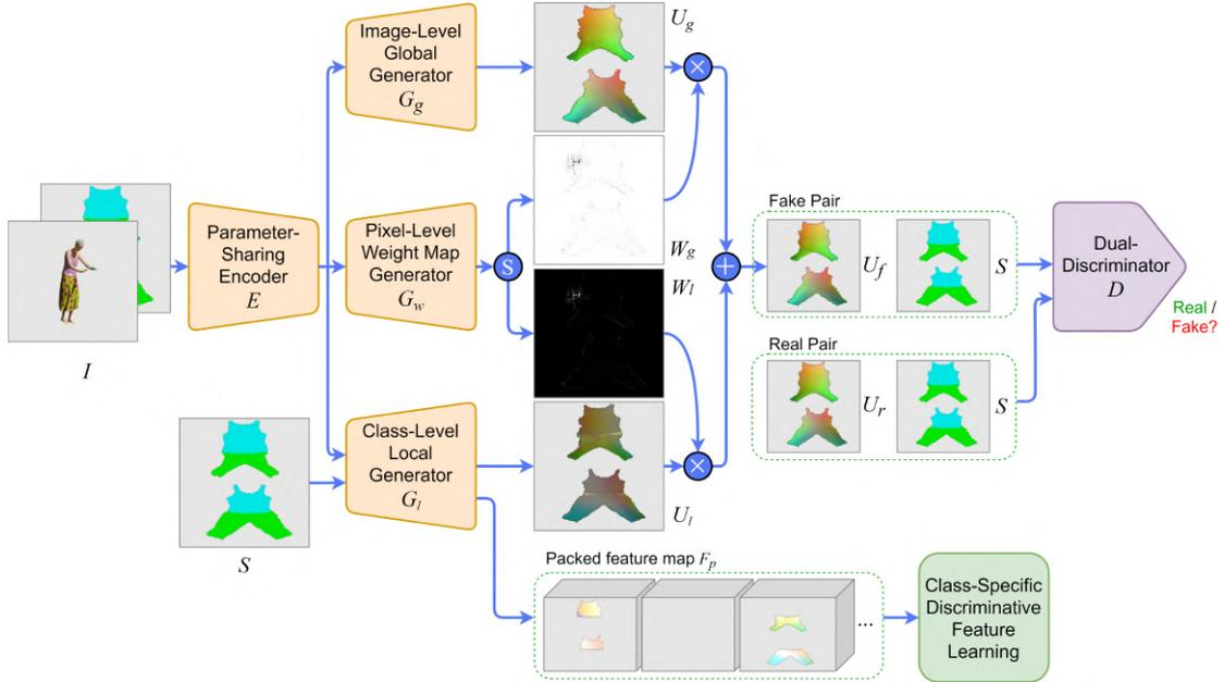
Figure 4.3: Overview of the proposed LGGAN. The symbol  $\oplus$  denotes element-wise addition,  $\otimes$  element-wise multiplication and  $\textcircled{S}$  channel-wise softmax. Source: Own elaboration adapted from [56].
