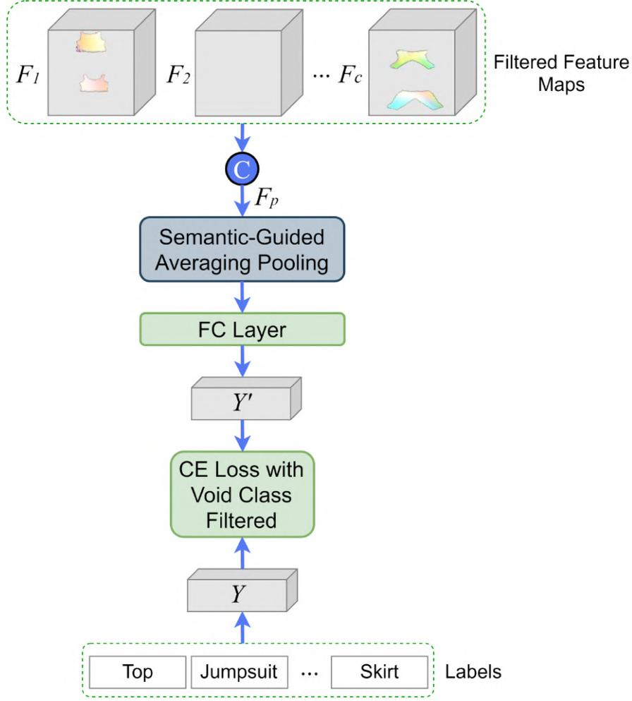
Figure 4.8: Class-Specific Discriminative Feature Learning architecture. Source: Own elaboration adapted from [56].
